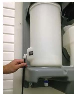
5. Install the fitting (thread sealant not included) you will need to connect to; a feed pump (push-in elbow fitting) or HydroDose (barb fitting) on the side port labeled "Chemical Outlet" and connect your tubing to the fitting. **IMPORTANT: Ball valve at the bottom of the unit is for a drain only. DO NOT draw chemical from this port.**
