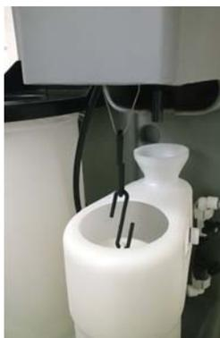
3. Install the float using both S-hooks. Verify that the float operation is not obstructed.
