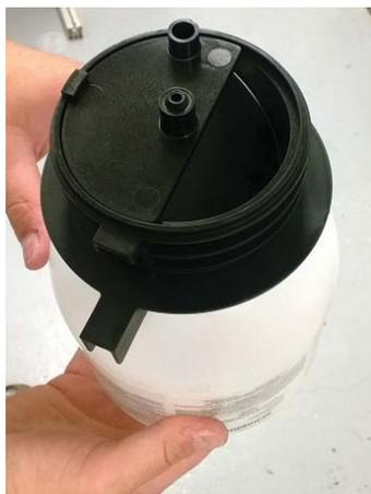
8. Remove the shipping cap and paper seal from the chemical jar.
