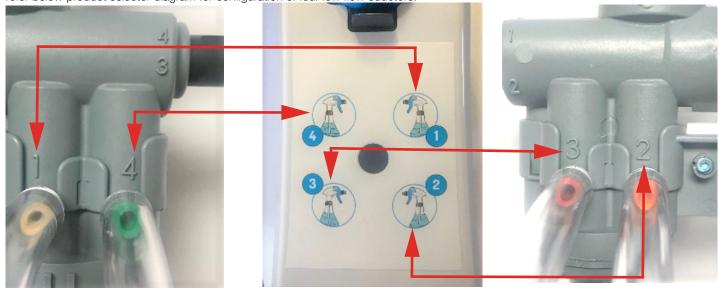
Location 4 is used to dispense water without chemical. The clear tip is installed in location 4 without drilling a hole on the tip. Refer below image.
