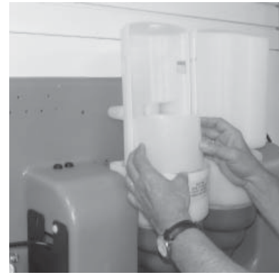
8. Stack chemical disks against back cover. Each disk holder will hold 4 disks. Replace the front covers.
