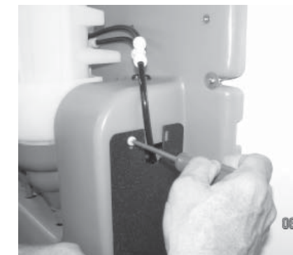
2. Remove both of the side access panels.
