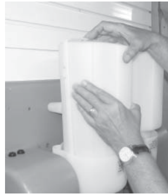
7. Remove the front covers from both disk holders.
