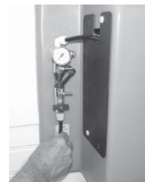
4. Connect water supply to the inlet ball valve push-in fitting.
