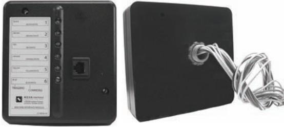
1. Route MI signal wires through 1/2 inch knock-out on washer (within the wiring area.)
