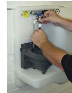
2. Install the siphon breaker by pushing the 1/4" fitting on the metal tube and the 3/8" fitting on the flexible black tube.
