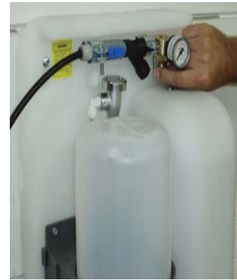
9. Turn on water supply valve. Adjust pressure regulator. 30-40psi is recommended.
