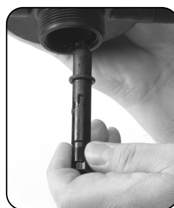
Step 6. Re-install #52 UPPER SHAFT and #17 O-ring.
