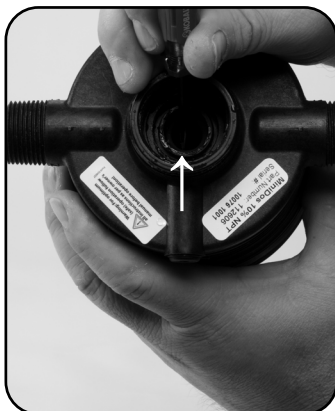
Step 4. Remove #17 O-ring and replace.
