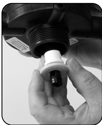
Step 7. Re-install #16 GASKET and #82 SEAL SPACER
