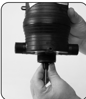
Step 8. Replace #51 SHAFT ASSEMBLY.
