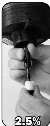
Step 2. Rotate #51 or #52 SHAFT 90° and remove.
