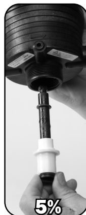
Step 2. Rotate #51 or #52 SHAFT 90° and remove.
