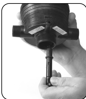
Step 5. Replace #17 O-ring.
