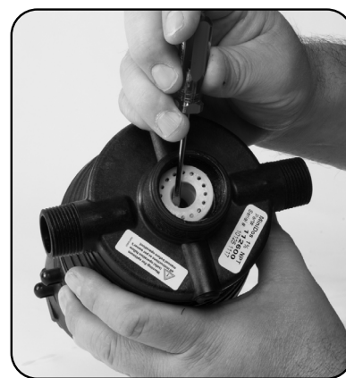
Step 3. Remove #16 Gasket.
