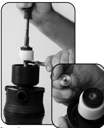
Step 2. Unscrew to unlock and remove #93 CAPSCREW.
