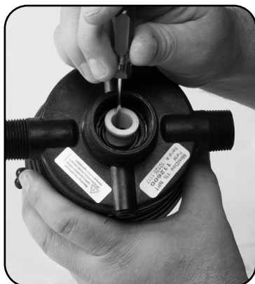
Step 4. Remove #82 SHAFT SEAL SPACER.
