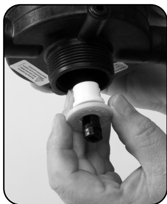
Step 7. Re-install #82 SEAL SPACER and #16 GASKET.
