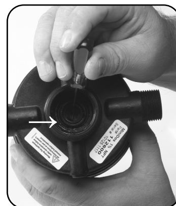
Step 6. Replace #17 O-ring.
