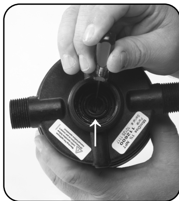
Step 5. Remove #17 O-ring and replace.
