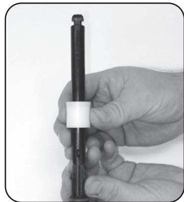
Step 4. For 2.5% & 5% Replace #44 DOSAGE PISTON flared-end up and #14 O-ring. 0.3% only: Replace #51 SHAFT ASSEMBLY. See Step 5a.
