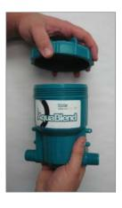
**Step 4.**Hold body firmly and unscrew the lid. If lid is tight, use 1' (25 mm) socket to loosen.
