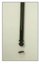
**Step 3.**Remove gasket from shaft. And install new one. If damage on sealing surface of shaft, replace shaft.
