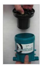
**Step 5.** Remove motor piston from pump body.
