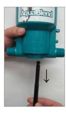
**Step 2.**Pull down on shaft, rotate shaft 90° and remove. Don't misplace tan gasket.
