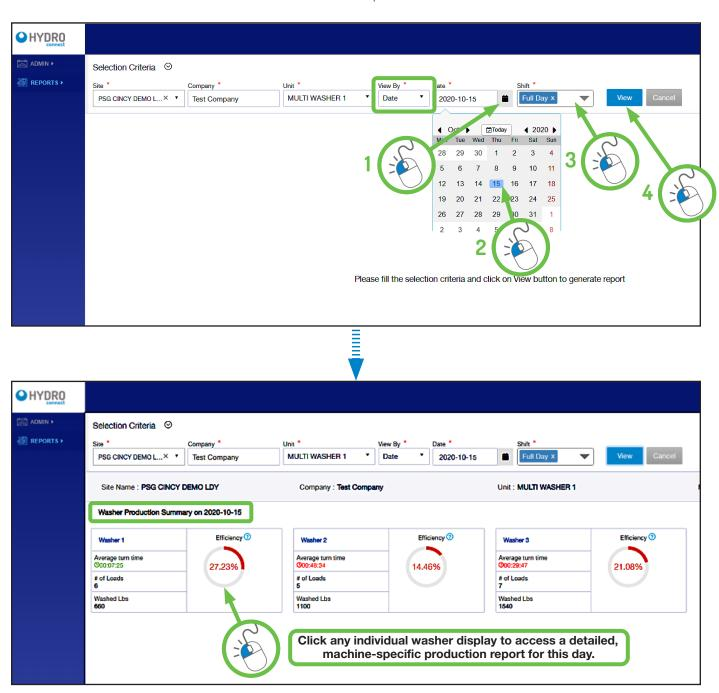
The resulting View By Date report (shown above) allows operators to see a summary of each washer in the facility with a breakdown of loads and weight run along with washer efficiency and average turn time on that date. (For more details, including the definitions of turn time and efficiency see the **Washer Production** section that starts on page 12.)
