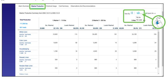
In the bar chart views, there is a control at the top-left side of the chart that allows the user to view either a total for the whole system or view one bar per washer.
