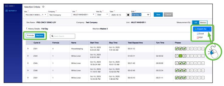
An operator can simply **click the down arrow** on the left side of the formula entry (as shown below) to expand the selection to show each individual product dosage; including the product dosed, the actual volume dispensed, and the time to do so.
