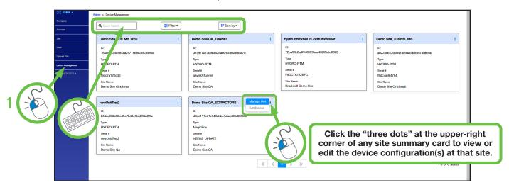
To view and edit the site configuration details remotely, **click the three dots** in the upper right-hand corner of the appropriate site card and select **Manage Unit**.
