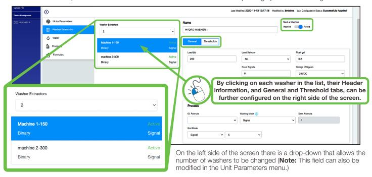
This is the **number of washers** configured with the Multi-Washer system and can be edited depending on the setup of the laundry. For MT10 Controllers the value can be set 1 to 10. For MT6, the value can be set 1 to 6.
