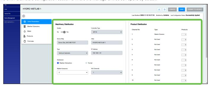
This section outlines the basic parameters of the dispensing system. Most of the fields in this section are not editable and are grayed out, indicating they are read-only. Each field is described in more detail below:
