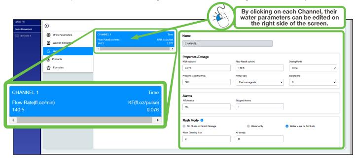
Toward the left side of the screen a list of "channel boxes" is displayed with a summary for each channel. The summary includes the channel name, pump mode, the calibrated flow rate, and the KF value from calibration. By clicking on each channel in the list, the parameters for water in the center of the screen can be set. Below is a description of each field:
