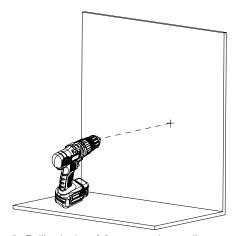
2. Drill a hole of 6mm on the wall at marked position.
