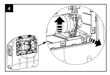
Lift the pump and remove clip securing pickup tube. WARNING TAKE CARE NOT TO DROP THE SECURING CLIP INTO THE WATER TANK.
