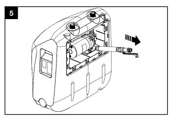
Remove hose using handle **WARNING TAKE CARE NOT TO DROP THE PICKUP HOSE INTO THE WATER TANK.**
