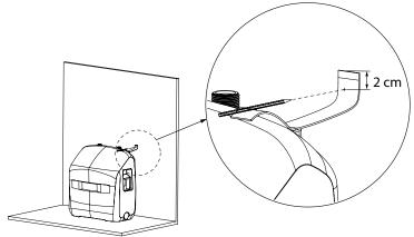
1. Place EvoBoost on a flat surface. Mark point on the wall to drill a hole.
