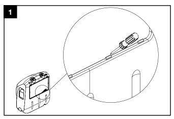
Remove Rear cover using flathead screwdriver to CAREFULLY pry the lower clips open.
