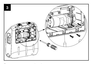
Remove screw securing the pump.
