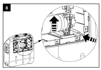
Lift the pump and replace securing clip back onto pickup tube WARNING TAKE CARE NOT TO DROP THE SECURING CLIP INTO THE WATER TANK.
