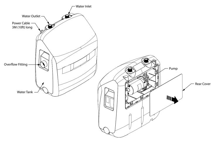
The EvoBoost is designed to supply laundry dispensers (max. 3 low flow EvoClean's) with 2.2 bar (32 psi) consistently with the EvoBoost installed, chemical delivery will be consistent and extremely accurate, leading to predictable laundry results. The key features of the unit are as follows:
