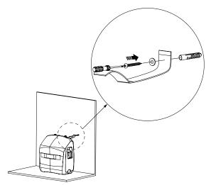
3. Install wall plug to the wall. Secure one end of strap to the wall with hardware using screwdriver.
