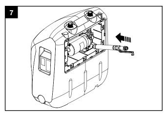
Clean inside of tank and lower the pickup tube back into the tank **WARNING TAKE CARE NOT TO DROP THE PICKUP HOSE INTO THE WATER TANK.**
