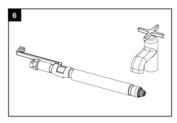
Clean pickup tube, removing any film, particles, dirt that may have built up.
