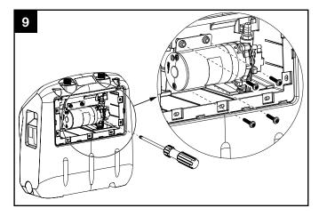
Secure the pump using screw.
