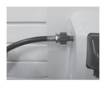
11. Connect water supply hose of at least 3/8" ID to water inlet swivel. Min. 25 PSI pressure is required for proper operation, Max. pressure 85 PSI and 120°F Max. water temperature. Connect opposite end of hose to water supply. Turn water supply on.
