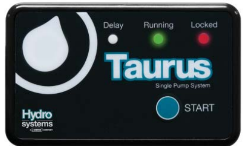
User Prime: Green LED stays on while yellow and red LEDs toggle with each press of START button (indicating User Prime enabled or disabled)
